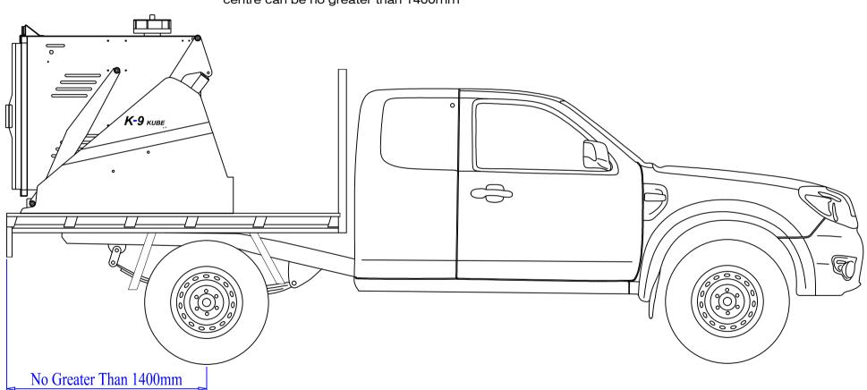
The overhang of the tray from the rear axle centre can be no greater than 1400mm
